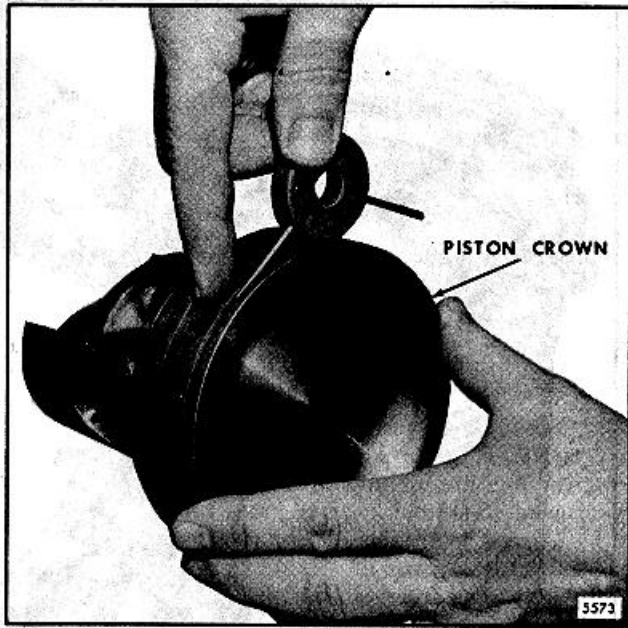
Fig. 5. Checking Fire Ring Groove in Piston Crown using Tool J 24599
