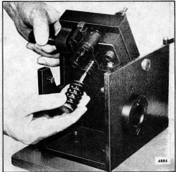
Fig. 24 Removing or Installing Plunger Follower, Plunger and Spring
