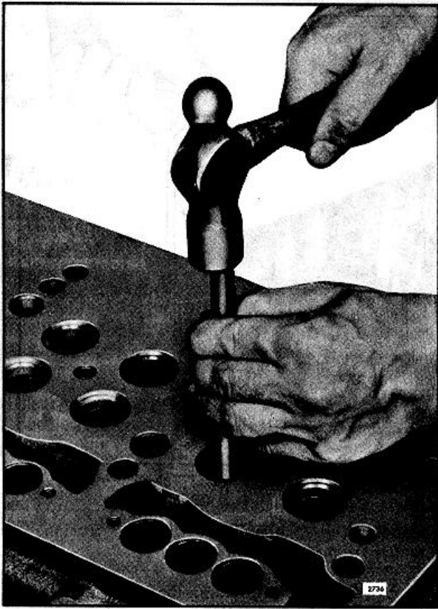
Fig. 6. Removing Exhaust Valve Guide
