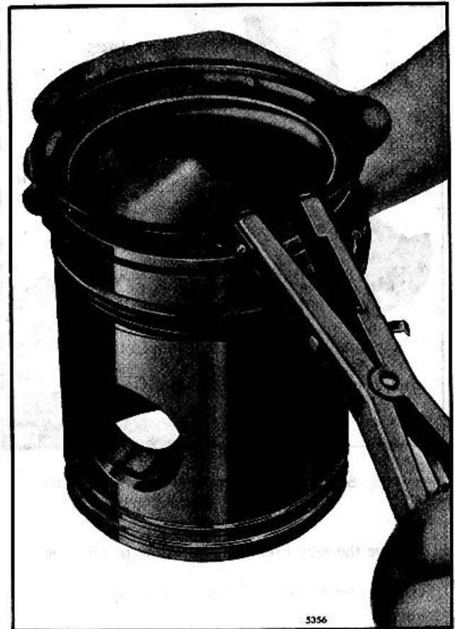
Fig. 4. Removing or Installing Piston Rings using Tool J 8128
